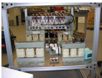
Low power and 5 MW PEBB, Variable voltage and frequency converter, & variable DC bus
