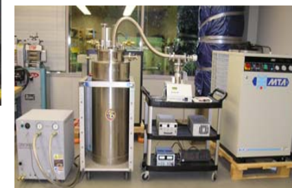
Superconductor AC Loss Msmt & Quench Stability & Propagation Test
